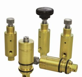
Regulators are offered in either relieving or non-relieving versions. The relieving design maintains a constant pressure output even when downstream conditions change, while non-relieving regulators do not automatically compensate for changes in downstream flow or pressure. There is no vent to atmosphere, as in a relieving type regulator, and the output pressure can increase due to a downstream event. Non-relieving versions can accommodate compatible liquid applications.
