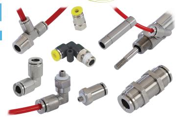
Constructed of high grade 316 stainless steel, these durable fittings provide a simple push-pull method of connecting pneumatic components to each other and system piping. Push-Quick fittings allow full flow through the hose/tubing I.D. with no smaller orifice required as in barb fittings. They are designed for use with both flexible hose and stiff tubing made of nylon, polyurethane, polyethylene or polypropylene. Many styles and sizes are available.
